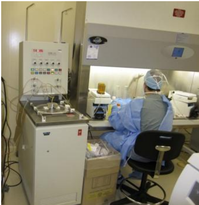
Gradient purification process using the COBE 2991 Cell Processor, separates the islets from the acinar cells
