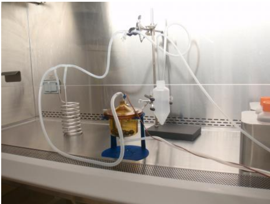
Media is heated up and circulated through the Ricordi chamber in this open loop system
